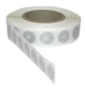
This NFC sticker is a 29mm diameter transparent sticky label that operates at 13.56 MHz wireless frequency and contains 137 bytes of usable read/write space for NDEF data. Based on the NTAG213 chip from NXP, this sticker offers advanced security, anti-cloning features as well as a permanent lock feature, therefore user data can be permanently configured read-only. The NTAG213 NFC chip features improved performance and is fully compatible with NTAG203 and MIFARE Ultralight C.
